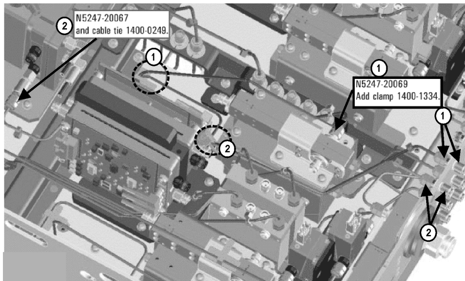
Figure 15 Location of Cable Clamp to Secure W41 and Cable Tie to Secure W55
